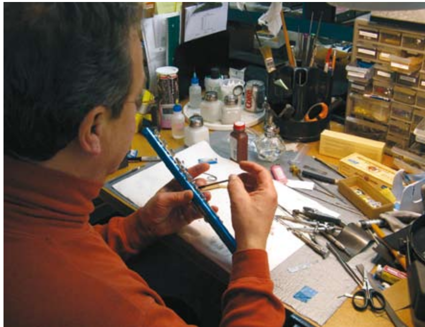
A flute being padded. The blue material has been stuck to the flute to preserve the finish while it is being handled.
