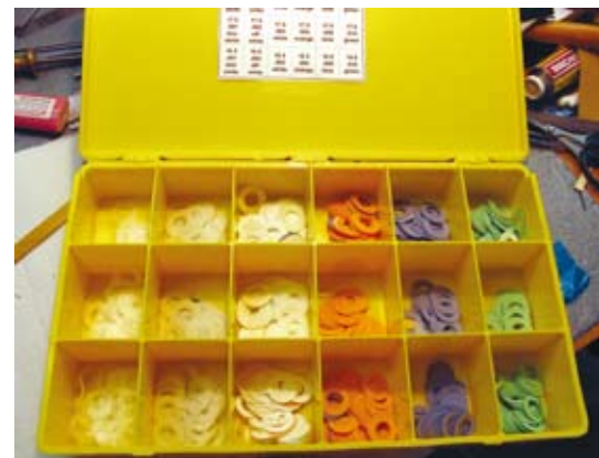
An assortment of paper shims used in padding a flute, colour-coded by diameter and thickness.
