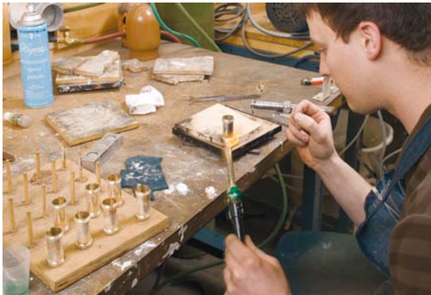
Soldering ferrules to a socket before soldering the socket to the flute body.
